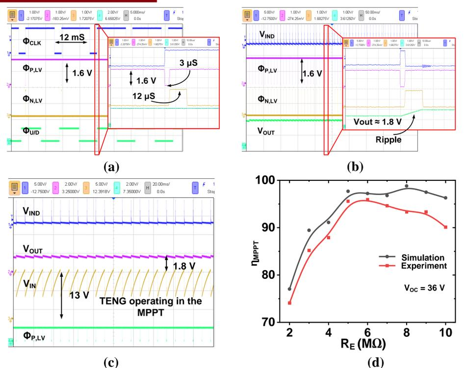
Fig. 4 Measured waveforms of the oscillator and MPPT controlling circuit, (b) inductor voltage (c) overall performance of the EHI-IC, (d) Tracking efficiencies as a function of the  $R_E$ .  $V_{OC} = 36$  V,  $R_{OUT} = 100$  k $\Omega$ .
