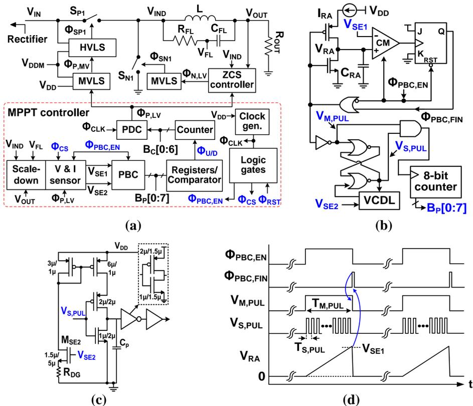
Fig. 2(a) Block diagram of proposed MPPT controller, (b) schematic of the PBC, (c) voltage-controlled delay line, (d) Operational waveforms of the PBC.
