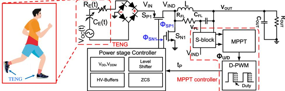
Fig. 1. Block diagram of proposed HV dc-dc buck converter.
